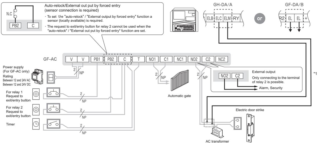
(\*1) The relay operating time of GH-DA/A (GF-DA/B) is different from that of GF-AC.
