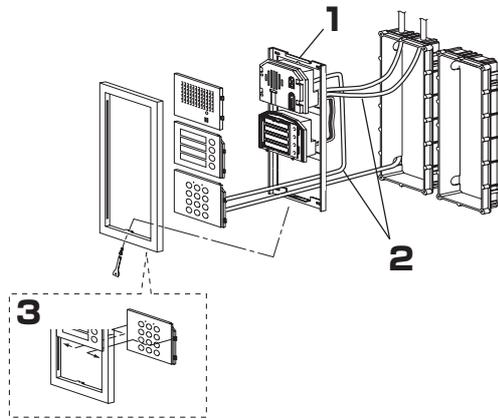
1. Fix the mounting bracket to the back (or surface-mount) box.
