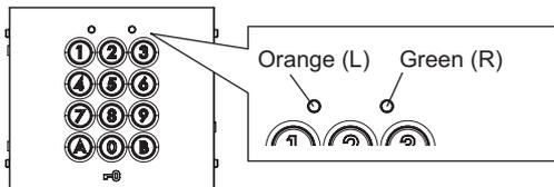
The result of each operation is indicated by the lighting up of the LED indicators on the upper section of the unit, and by the sounding of the buzzer.
